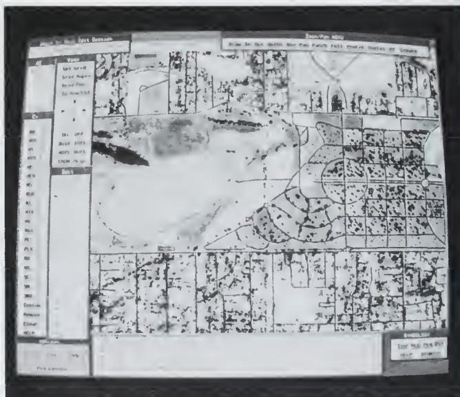
Figure 14. On the left, an orthophoto enlargement produced from 1:40,000 scale NAPP aerial photograph. The cadastral survey landnet registers to the image because the image was scale and displacement corrected. On the right, a digital orthophotoquad is displayed on a workstation for automated map update and maintenance.
